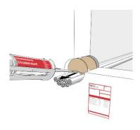
**ZZ®** 345 Fire Protection Silicone must be introduced uniformly into the opening from back to front. The gaps should be filled with sufficient sealant.
