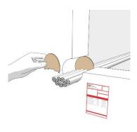
Backfill material, consisting of mineral wool, cardboard or polyethylene can be used. It must be ensured that the minimum fill depth of the
