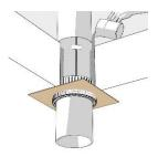
**ZZ**<sup>®</sup> **430 Fire Protection Collar** for ceiling installation, it must be mounted on the underside. The use of formwork is particularly suitable for this purpose.
