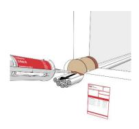
**ZZ**<sup>®</sup> 333 Fire Protection Mastic must be introduced uniformly into the opening from back to front. The gaps should be filled with sufficient sealant.
