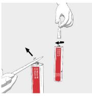
Hold the cartridge vertically, cut off the tip with a sharp knife, and screw on the nozzle. The nozzle can be shortened as needed.
