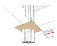
For larger openings in floors the use of a formwork on the underside of the floor is recommended. This can remain on the through penetration firestop system.
