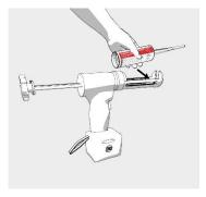
Insert the cartridge into the dispensing gun.
