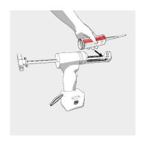
Insert the cartridge into the dispensing gun.
