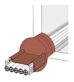
The beginning and end of the **ZZ® 451 Fire Protection Bandage** must be connected with at least two steel clips or steel wire. The length of overlap must be at least 45 mm.
