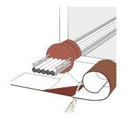
Cut off a sufficiently long piece of **ZZ® 451 Fire Protection Bandage** and after removing dirt from the installation, peel off the protective film and apply the bandage. For wall mounting, apply on both sides, and for ceiling mounting, apply it on the upper side of the ceiling.
