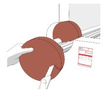
**ZZ® 130 Fire Protection Plug.** for the component opening and cut them to the appropriate size for the penetrating elements.
