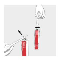
Hold the cartridge vertically, cut off the tip with a sharp knife, and screw on the nozzle. The nozzle can be shortened as needed.
