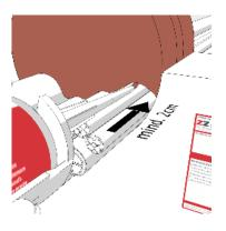
Interstices between cables and open joints must be filled with **ZZ® 333 Fire Protection Mastic** at least 20 mm deep on both sides.
