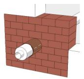
The beginning and end of the **ZZ<sup>®</sup> 451 Fire Protection Bandage** must be connected with at least two steel clips or steel wire. The length of overlap must be at least 45 mm.
