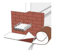
Cut off a sufficiently long piece of **ZZ<sup>®</sup> 451 Fire Protection Bandage** and after removing dirt from the installation, peel off the protective film and apply the bandage.
