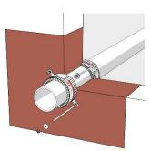
For wall mounting, apply **ZZ<sup>®</sup> 430 Fire Protection Collar** on both sides. Therefore the same threaded rods can be used for both sleeves.
