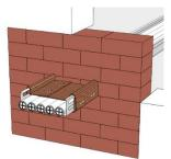
For wall mounting, apply **ZZ<sup>®</sup> 451 Fire Protection Bandage** on both sides, and for ceiling mounting, apply it on the upper side of the ceiling.
