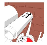
Interstices between cables and open joints must be filled with **ZZ<sup>®</sup> 333 Fire Protection Mastic** at least 20 mm deep on both sides.
