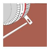
Pass the Ø6 mm threaded rods through the penetration and secure **ZZ<sup>®</sup> 430 Fire Protection Collar** with washers and nuts.
