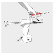
Insert the cartridge into the dispensing gun.
