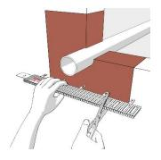
Select the suitable collar size for the pipe or cut the **ZZ<sup>®</sup> 430 Fire Protection Collar** to size.
