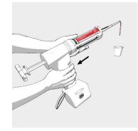
Start pressing out **ZZ® 330 Fire Protection Foam** and discard non-uniform initial material.
