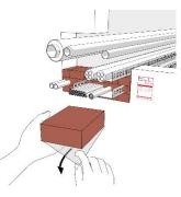
Install the **ZZ® 230 Fire Protection Block** snugly in the masonry bond within the component opening, after removing the protective film.
