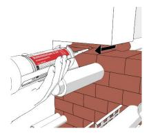
**ZZ**<sup>®</sup> **330 Fire Protection Foam** should be worked into the opening from back to front. In this process build up the foam from bottom to top, always guide the tip of the mixing nozzle above the foam so that the material does not stick or clog. If work is interrupted for more than 50 seconds the foam will harden in the mixer.
