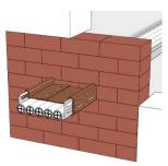
The beginning and end of the **ZZ® 451 Fire Protection Bandage** must be connected with at least two steel clips or steel wire. The length of overlap must be at least 45 mm.
