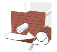
Cut off a sufficiently long piece of **ZZ**<sup>®</sup> **451 Fire Protection Bandage** and after removing dirt from the installation, peel off the protective film and apply the bandage. For wall mounting, apply on both sides, and for ceiling mounting, apply it on the upper side of the ceiling.
