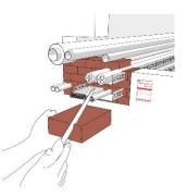
Cut the **ZZ<sup>®</sup> 230 Fire Protection Block** to the size of the exposed area.
