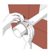
Place the **ZZ® 430 Fire Protection Collar** around the pipe. Fasten the fire protection collar by pulling the locking tab through the opening and bending the tab 180°.
