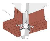
**ZZ**<sup>®</sup> **430 Fire Protection Collar** must be installed on the underside for ceiling mounting.
