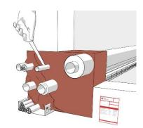
Trim any excess **ZZ® 330 Fire Protection Foam** with a suitable knife after approximately 2 minutes, observing the necessary safety precautions and regulations.
