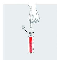
Hold the cartridge vertically with the tip pointing upward, unscrew the sealing cap and screw on the mixer provided.
