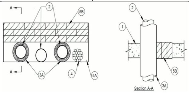
1. **Floor or Wall Assembly** — Min 4-1/2 in. (114 mm) thick reinforced lightweight or normal weight (100-150 pcf or 1600-2400 kg/m $^3$ ) concrete. Wall may also be constructed of any UL Classified **Concrete Blocks\*.** Max area of opening is 384 in. $^2$  (2477 cm $^2$ ) with a max dimension of 32 in. (813 mm).
